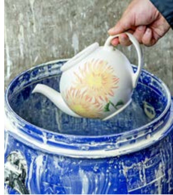
Following the biscuit firing, a teapot is dipped into a barrel of glaze to ensure it is fully coated.
