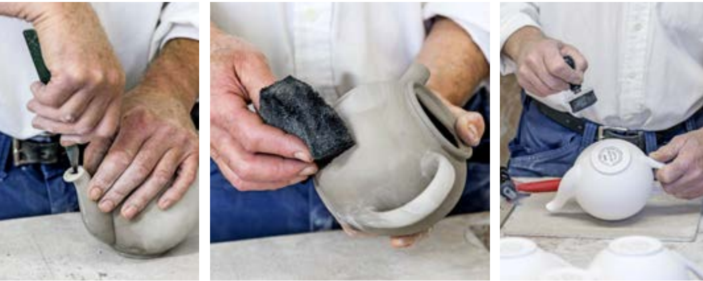
Left to right: Opening the spout with a sharp knife; roughening the teapot's surface with a sponge to better apply the paint; stamping the pottery logo onto the base of the pot.
