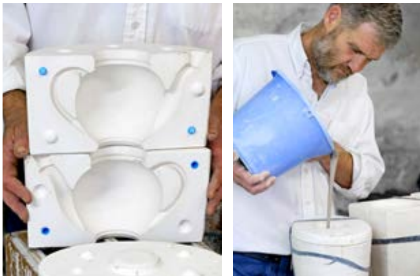
The two halves of the reusable plaster mould for making a teapot.
