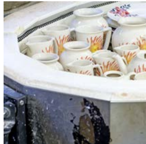
Glazed pottery cooling in the kiln, after firing at a temperature of more than 1,000°C.
