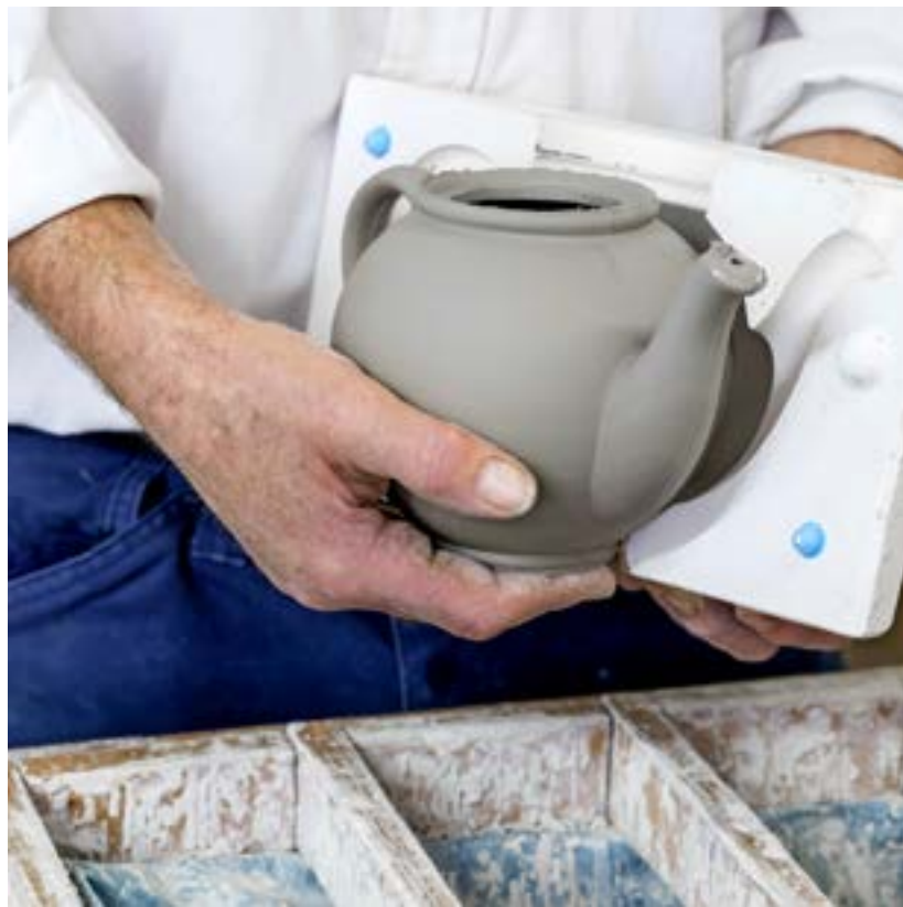
The two halves of the reusable plaster mould for making a teapot.
